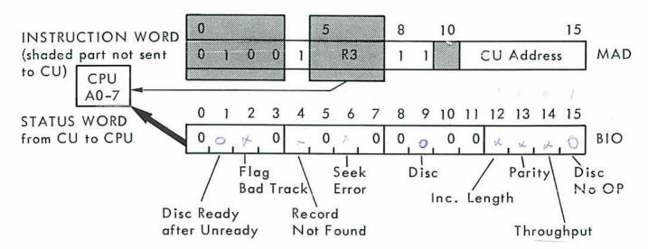
The SST instruction is used to transfer the CU status word to the CPU accumulator specified by the R3 field. SST is accepted by the CU if the CU is in Wait-Status state.
