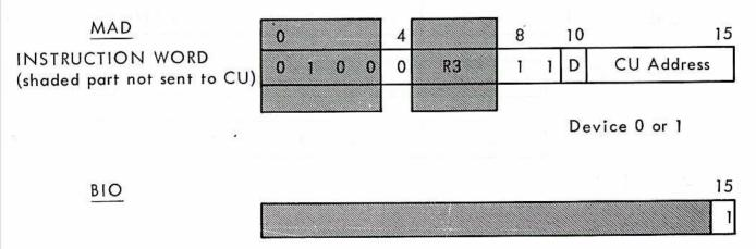
A special CIO Start/IPL instruction is used to transfer an Initial Program Loader (IPL) from the disc to the memory. The IPL is assumed to be already located on
