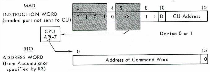
The CIO Start instruction is used, after a group of commands has been programmed in the main memory, to begin CU operation. The CIO Start is accepted if the CU is not already performing an operation on the addressed disc unit.
