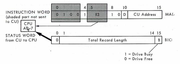
This command is used before an I/O operation to test if a disc drive is busy, or following a Read operation to obtain the total length of the record that was read. The TST command is always accepted by the CU. Upon receipt of this command, the CU puts the drive status and the record length on the BIO lines, as shown above.
