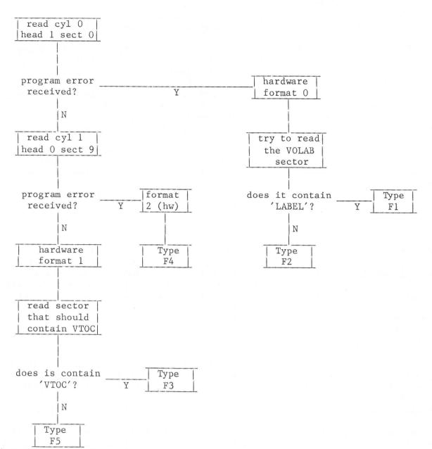
A program error is returned by the control unit, if an access is made to a nonexisting track or to a non-existing sector (i.e a too high sector number). So the first check on program error determines whether there are one or two tracks (surfaces) available on a cylinder and the second check whether there are 8 or more (so 26) sectors available on the track. These two checks identify fully the hardware format.
